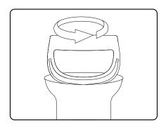
(2) Unscrew and remove the pump by turning the handle in an anti-clockwise direction.
