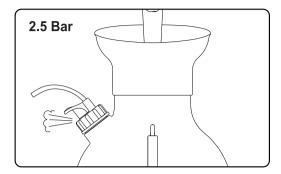
9 Ensure that pressure is released and that all sprayer components are rinsed thoroughly with water after use. This can be achieved by filling the bottle with clean water, pressurising and then emptying via the nozzle. Clean after every use and do not store liquids in the unit.
