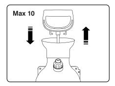
5 Pressurise the bottle by pumping the lever up to 10 times. Do not over pressure.
